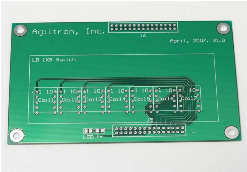
Fig. 2: Layout of evaluation kit switch board
