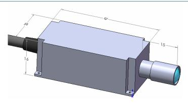
2000 nm isolator collimator example
